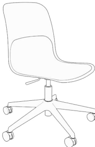
5 Star Aluminium base with castors and height adjustable seat plate.
