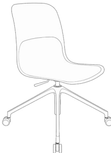
Height Adjustable 4 Star Aluminium base with castors and height adjustable seat plate.
